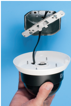
2 Place assembly on bracket. Turn clockwise to lock. Install set screw.
