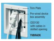
2 Attach device box to trim plate with screws provided. Secure trim plate to wall with mounting wing screws. Install CED130 in 2-gang boxes. Pull cables.
