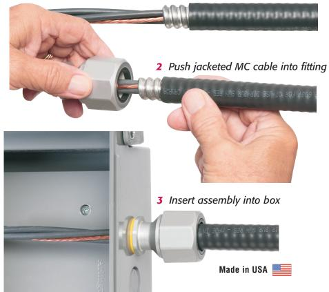
Save time and money with Arlington's liquid-tight, concrete-tight fittings designed especially for PVC jacketed MC cable - and Teck 90 cable.
