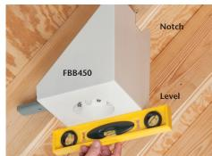
NO need for a 2x8 or extra trimming! Notch the box as necessary, keeping bottom of box level - with short side of box touching rafter. Screw the bracket to the rafter with (4) supplied #10, 1-1/2" wood screws through the pre-drilled screw hole(s) in bracket.
