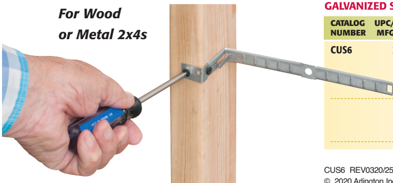
4 Bend tab over support to lock cable securely in place. CUS6 holds up to FOUR MC cables – or SIX NM Cables centered on a 2x4.
