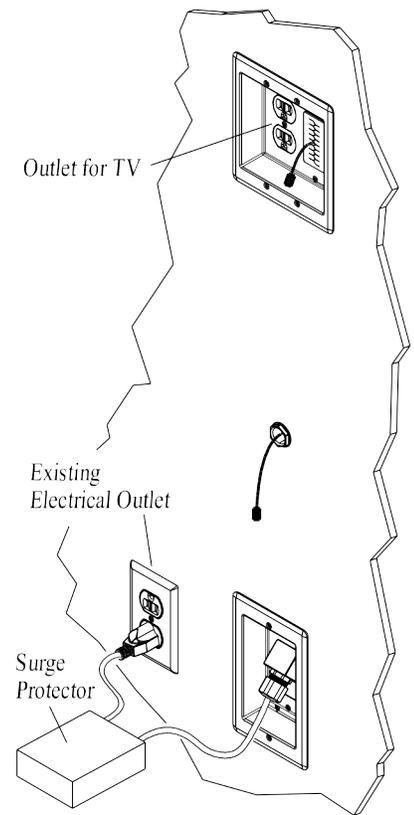
View of Completed Installation of TVBRA3K Pre-Wired TV Bridge
