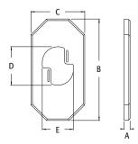
Use the 8100LP to convert octagonal size covers to MEGA covers for mounting large fixtures or coach lamps. UV rated plastic for long outdoor life.
